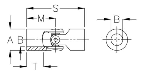
$\begin{array}{lll} A & = 63 \\ B \ H7 & = 40 \\ M & = 83 \\ MD \ max \ N \ m = 250 \\ s & = 166 \\ T & = 50 \\ \end{array}$
